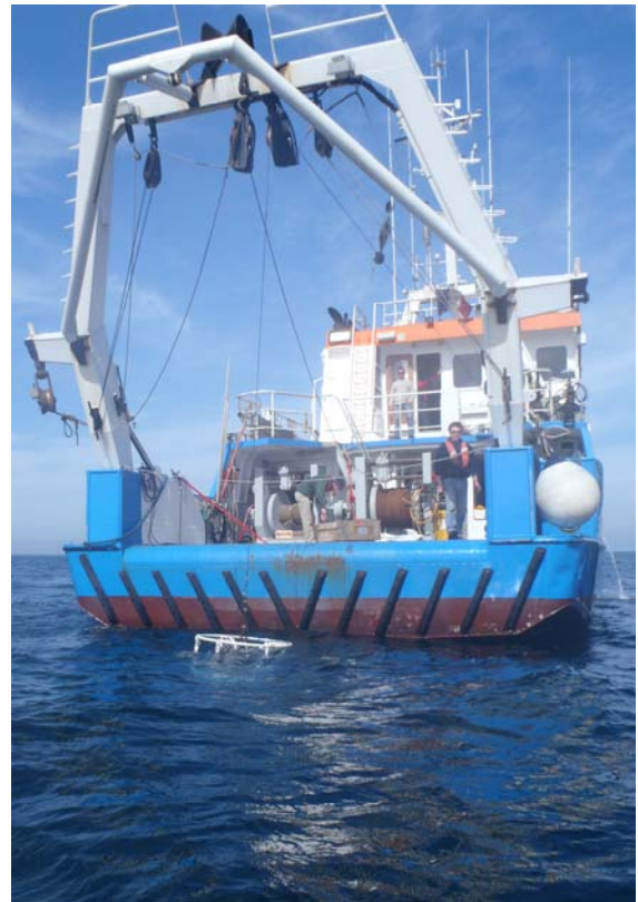
The beginning of a CTD cast with water sampling in the vicinity of the BOUSSOLE buoy.
